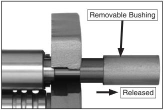
Figure 31. Removable bushing release (T21324 shown).
